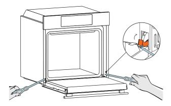
2. To refit, place door back onto the hinges and use a screwdriver to rotate the hinge locks back into the hinge cavity.
