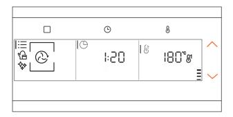
2. Press  $\checkmark$  or  $\land$  to scroll through the COOKING FUNCTIONS menu and select the desired cooking function.
