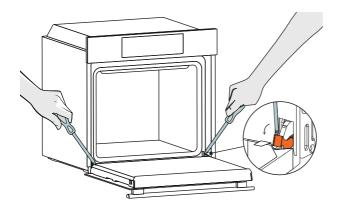
1. Open the door fully and use a screwdriver to rotate the hinge locks outwards, then carefully lift the door off and place it on a soft, level surface.
