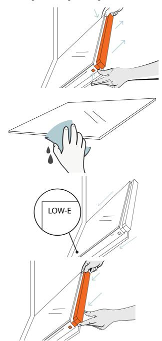
1. Shut the door halfway, then press the buttons on both sides of the door at the same time to release the cover on top of the door.
