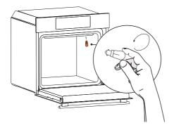
2. Unscrew the light bulb to remove it. Replace with a new bulb and refit the protective cover.
