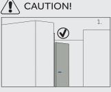
When you close the door, the vertical door strip on the left door should be bent inside (1).
