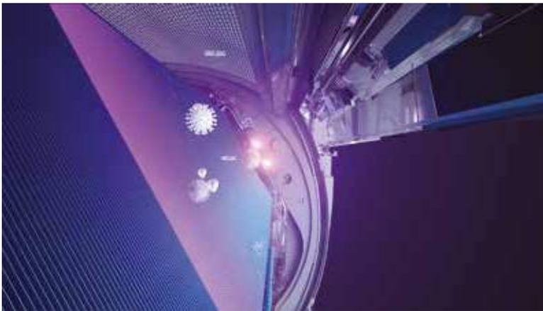
The Haier air conditioner is equipped with a UVC generator module, which uses UV light to eliminate airborne hazards staphylococcus aureus bacteria at 92.78% effectiveness, and H3N2 virus at 91.47% effectiveness\* as they pass through the unit.
