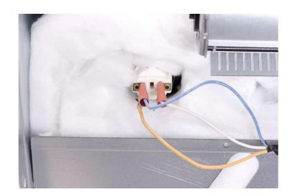
Pull and remove the cables attached to the lamp located behind the chassis from their terminals to replace the oven lamp. You can remove the lamp cleared off the cable connections by pressing the tabs.
