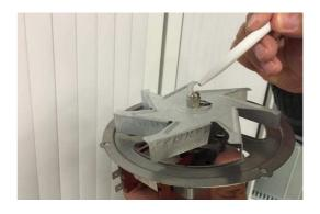
Remove the closed bolt to remove the propeller.
