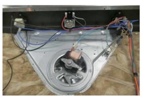
Remove the cables connected to the safety thermostat with a socket by holding on the terminals.
