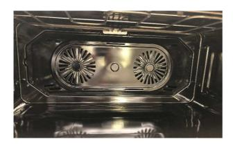
There are four screws holding the fan protection sheet in the chassis.
