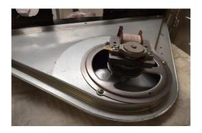
Remove the screws that connects to cooling duct.
