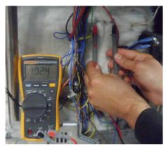
If any value appears on the multimeter screen, it means the heating element is in operating status.
