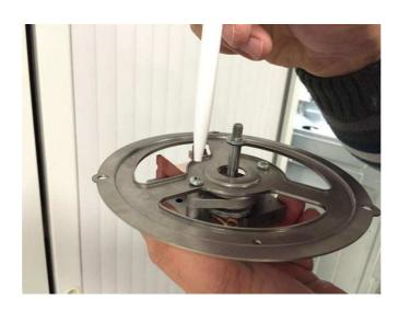
Remove the propeller before removing the motor assembly.
