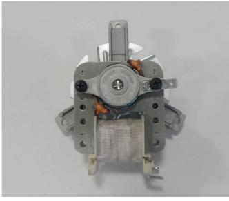
Remove the turbo motor by removing the screws.
