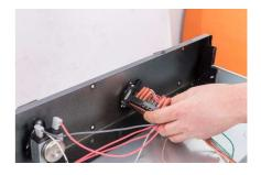
Remove the circuit breaker shell by turning it right or left.
