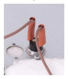
The purpose of the safety thermostat is cut off the phase or neutral before the oven temperature exceeds a certain value when the thermostat on the oven is short-circuited or due to continuous operation of any heater resulting from a short circuit. Since the point where the thermal cutter fitted on the oven is taken as the reference, the safety thermostat is expected to switch off only under abnormal conditions but not under normal conditions.
