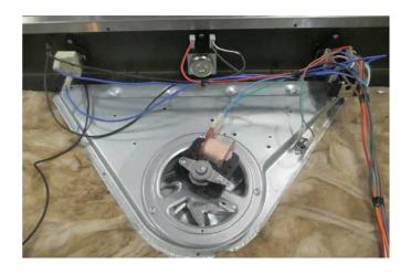
You can access circuit breaker, thermostat, mechanical/digital clock and cable connections after removing the service cover.
