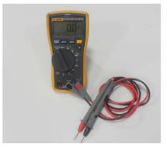
Multimeter set to heating element measuring position to measure the heating element value. If the heating element is OK, a heating element values appears on the multimeter.
