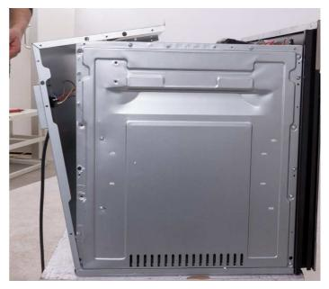
Remove the screws on the rear guard of the oven with a screwdriver.
