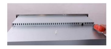
Remove the screws that connect the service cover of the product to the top cover.
