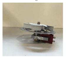
This fan is located on the upper section of the oven cavity. It gets activated directly when the oven is started. It is deactivated by means of a second safety thermostat. It prevents oven from getting overheated and protects control panel section against heat and humidity.
