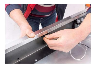
Signal light is attached to the signal light plug located behind the panel with a socket. Pull and remove the socket. Fit the new signal light on the place of the old one in the switch.
