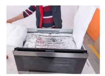
Remove the wire of the insulation coiled around the chassis with wire.
