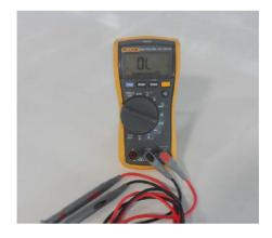
If no value appears on the multimeter display, it means that the heating element is defective.
