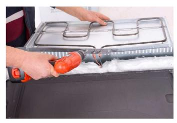
Remove screws with the help of screwdriver and remove cables on the heating element. Push from sides of heating element cover plate and pull towards back side of oven as shown in picture.
