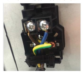
The mains cord connection on all the appliance where small terminal box is used must be made as shown in the image.
