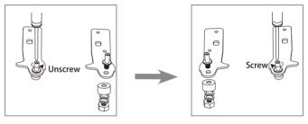
7. Refit the bracket fitting the bottom hinge pin. Replace the adjustable foot.
