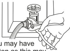
2. Connect the water inlet hose to the water faucet. You may have to use pliers to tighten the coupling. Do not over tighten as this may cause damage to the valve or hose fittings.
