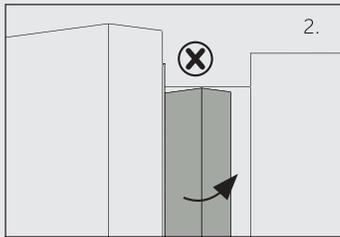
If you try to close the left door and the vertical door strip is unbent (2), you should bend it firstly, otherwise the door strip will hit the fixing shaft or right door. Thus a damage to the door slip or a leak will occur.
