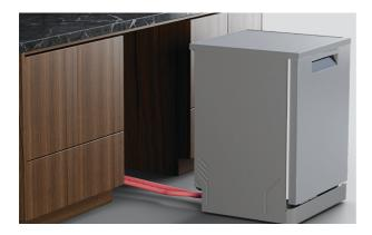
2. Push the product into the position, pulling the hoses through as you push to avoid crushing or twisting them. Take care not to bend the legs.
