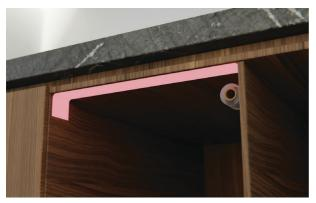
**3.** Align the supplied moisture protection tape to the cabinetry as shown.
