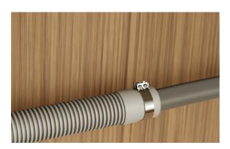
2. Pull the hose through the drain hose support before threading the hose clamp onto the hose and fitting to the sink trap. Secure to trap using the clamp. Ensure hose is routed straight to the trap.
