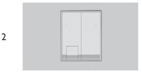
Using the template as a guide, pre-drill all holes into the panel.
