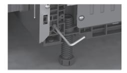
Use a 4mm Allen key to adjust the door tension. Rotate clockwise to increase tension, rotate counterclockwise to decrease tension.
