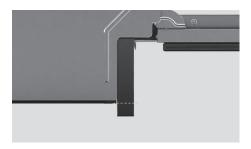
Align both sound seal sheets to the base of the dishwasher. If required, trim excess felt.
