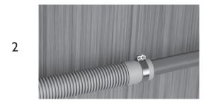
Pull the hose through the drain hose support before threading the hose clamp onto the hose and fitting to the sink trap. Secure to trap using the clamp. Ensure hose is routed straight to the trap. Unplug or drill out the waste tee before securing joiner to sink trap or waste tee.
