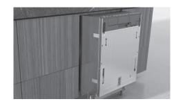
Select desired spacer width and cut to size. Remove adhesive and fit two spacers to each side of the product. Push the product into the cavity from the outside edges.
