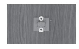
Ensure the sliding bracket is oriented correctly before securing it to the panel.
