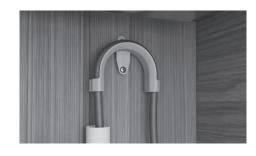
Pull the hose through the support guide and rest in standpipe. Ensure the drain hose does not extend
