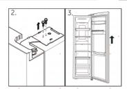
2.Undo the screws holding the upper hinge in posi-tion and then remove the hinge.3.Lift the freezer conpartment door to remove it.
