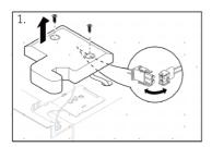
1.Undo the hinge cover screw and remove the cover. Release the cable connector.
