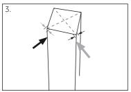
3. The stability can be checked by alternately bumping on the diagonals. The slightly swaying should be the same in both directions. Otherwise the frame can warp; possible leaking door seals are the result. A low tendency to the rear facilitates the closing of the doors.
