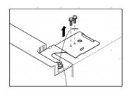
4.Refit the door by reversing the removal steps. Ensure that the grounding cable will be fixed by the screw.
