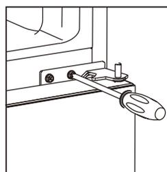
4. Laying down the refrigerator, take out the adjusting feet as below, then unscrew the lower hinge by cross screwdriver.
