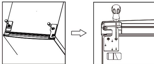
Unplug the temperature sensor from inside the top hinge cover and put the sensor back into the unit as shown below. Remove the door carefully and safely place to protect it from damage.
