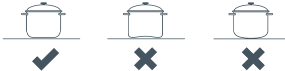
Fig. 15 Efficient and inefficient saucepan bottoms
