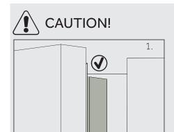
When you close the door, the vertical door beam on the fridge left door should be bent inside (1).
