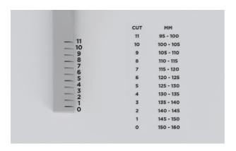
1. Measure the distance between the floor and the base of the door. Refer to the table and mark out the cut location.
