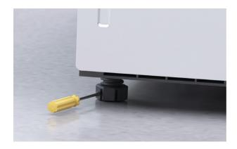
1. Using a flat bladed screwdriver, turn to raise the leveling feet. Level the rear, outside legs first followed by the front legs. Do not adjust the rear middle leg yet.
