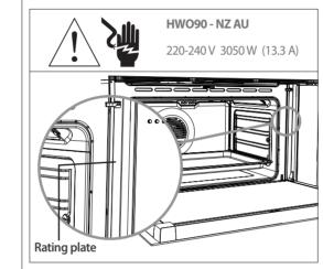
Connecting the oven to the mains power supply
