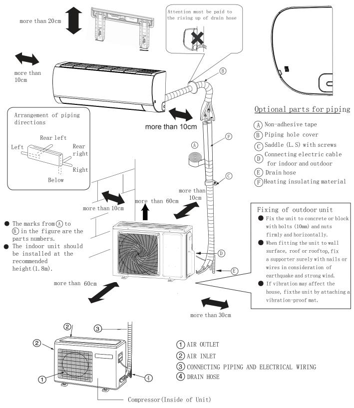
1. When installing the unit to wall, roof or rooftop, fix a supporter surely with nails or wires in preparation of earthquake and strong wind. 2. Air conditioner mounted not above and one meter away from electric equipment such as television.
