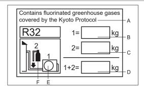
This product contains fluorinated greenhouse gases covered by the Kyoto Protocol. Do not vent into the atmosphere. Refrigerant type: R32
