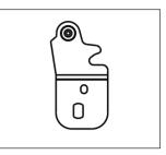
8. Refit the bracket fitting the bottom hinge pin. Replace both adjustable feet. Transfer the lower door to the property position.
