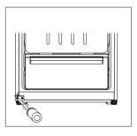
Make the middle hinge reverse the direction 180°C, then transfer it to the left property position. Make the middle hinge pin in the upper hole of the lower door, then tight the bolts.
