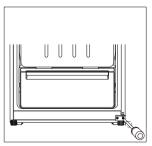
7.Disassemble right hinge, find out left bottom hinge from spare parts bags and fix it.
