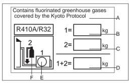
This product contains fluorinated greenhouse gases covered by the Kyoto Protocol.Do not vent into the atmosphere.
