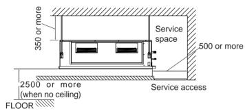
(2) Installation by which service is carried out from the bottom of the unit
