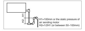
Taking the ADH\*\*H serials as an example, the installation of the drain pipe is the following.
